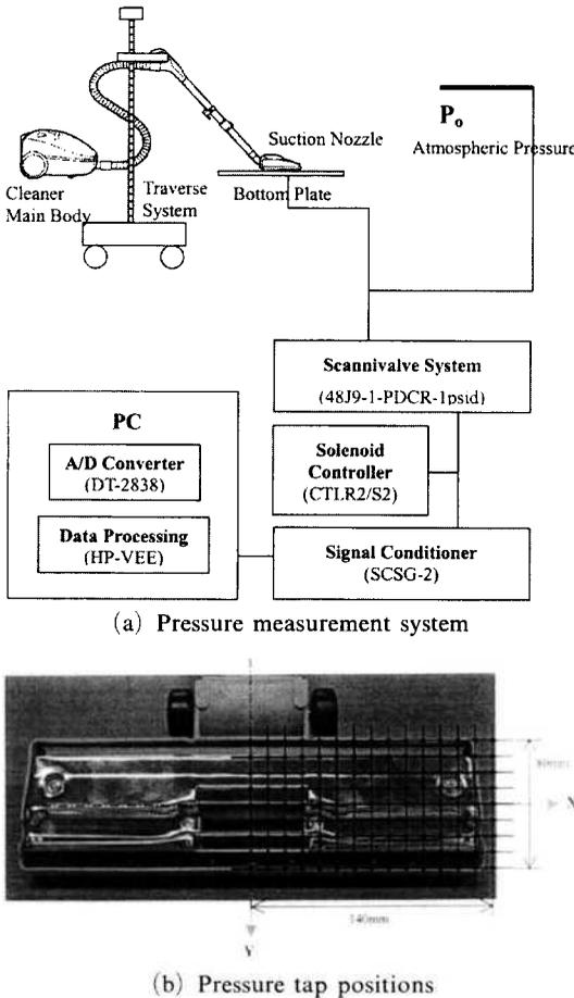
Fig. 2 Schematics of suction pressure measurement system and pressure tap positions on a flat bottom plate
