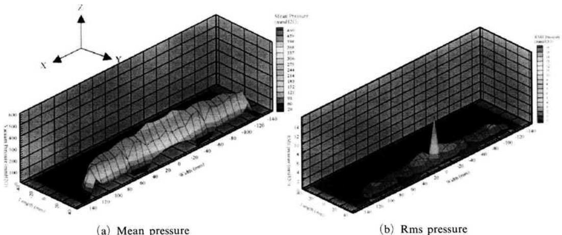
Fig. 7 Suction pressure distribution for connecting chamber modification
