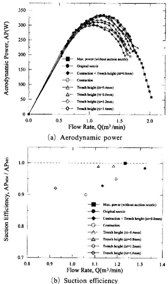
Fig. 4 Aerodynamic power and suction efficiency for modified suction nozzles over an artificial lawn
